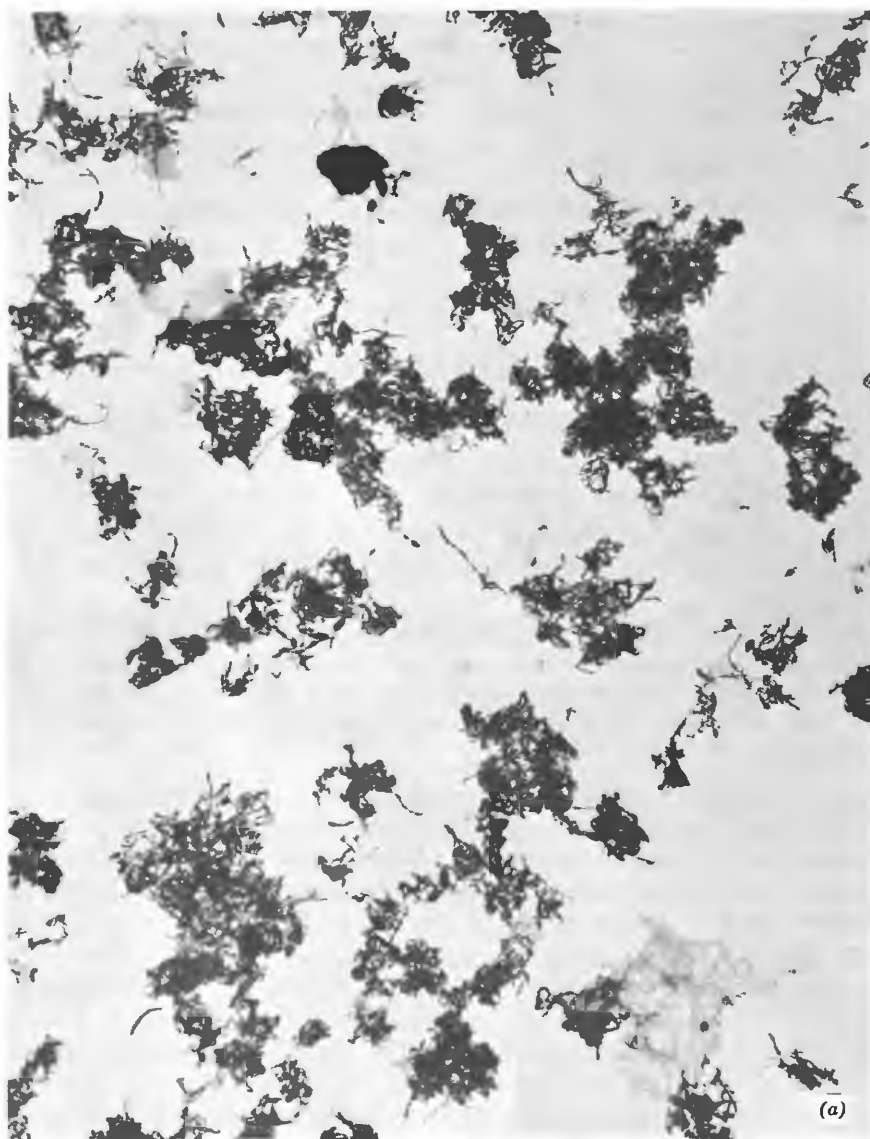
Figure 4. Filamentary silver produced by Developer D-76 (a) compared to silver given by a mercaptoacetic acid monobath (b). The anti-physical-developing activity of the potassium hydroxide-mercaptoacetic acid monobath has produced finer silver filaments than those given by the high-sulfite D-76 developer (10,000 \times ). (Grant Haist and James King, Eastman Kodak Company).
