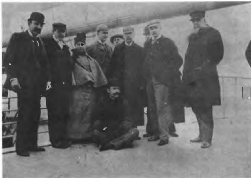
Figure 9. Restoration of faded photograph through the use of sodium borohydride solution. Only the left half of this old photograph, mounted on card, was swabbed with the borohydride solution to show darkening of the image. (From the author's collection)
