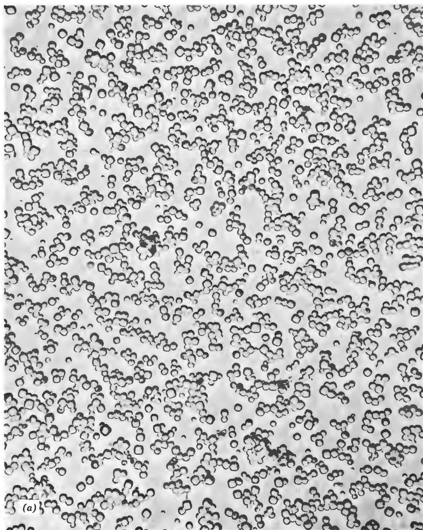
Figure 2. The incorporated chemical film contained both the developing and stabilizing compounds in the silver chloride emulsion layer: (a) the shadowed replica of the emulsion grains (15,000 \times ), (b) the form of the processed silver of a maximum density area (22,500 \times ). Processing consisted of heating the back of the photographic material for 15 sec at 160°C, causing both development and stabilization to occur. (Grant Haist, Eastman Kodak Company)
