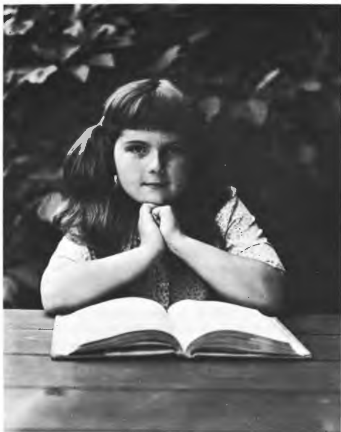
Figure 1. Proof contact print of negative of Lynne Haist made on experimental photographic paper containing both developing and fixing compounds in the emulsion layer. The exposed paper was immersed for 10 sec in a simple alkaline activator at 75°C, then washed briefly in water. Print is 11 years old. (Grant Haist, Eastman Kodak Company)
