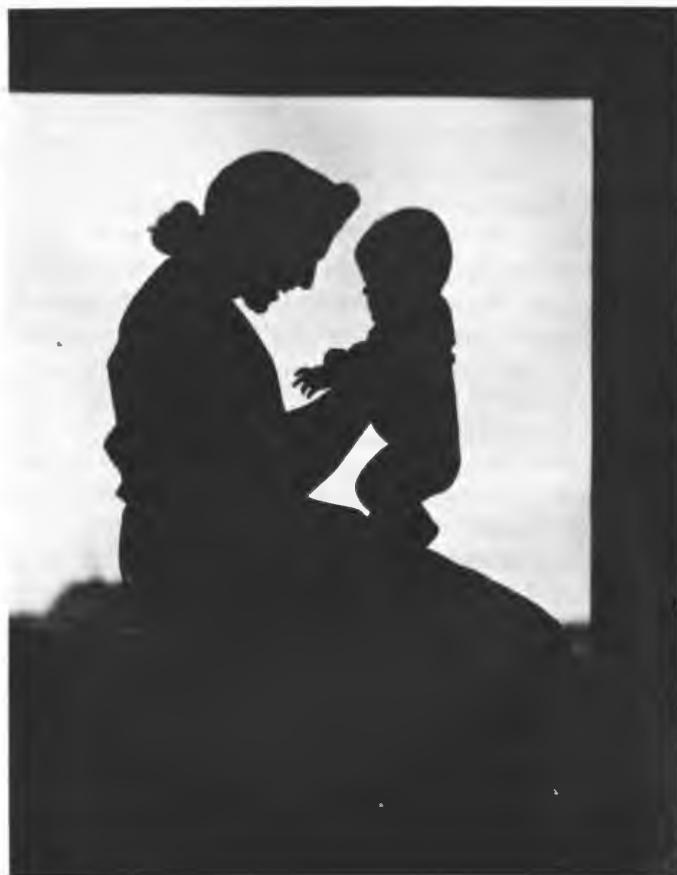
Figure 2. Contact print made on an experimental paper containing both developing and stabilizing compounds in the emulsion layer. The exposed paper was thermally processed by contacting the back of the print for 30 sec on a metal platen heated to 180°C. The stabilized print has not changed in 15 years of room storage. (Grant Haist, Eastman Kodak Company)
